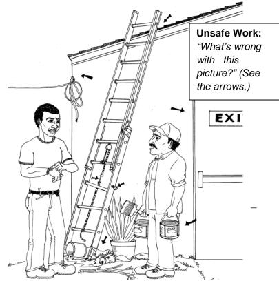
*Joe:* This bolt seems a bit loose, and the pulley rope is a bit frayed. I wonder how that happened...and the steps feel like they have some kind of slippery stuff on them...
