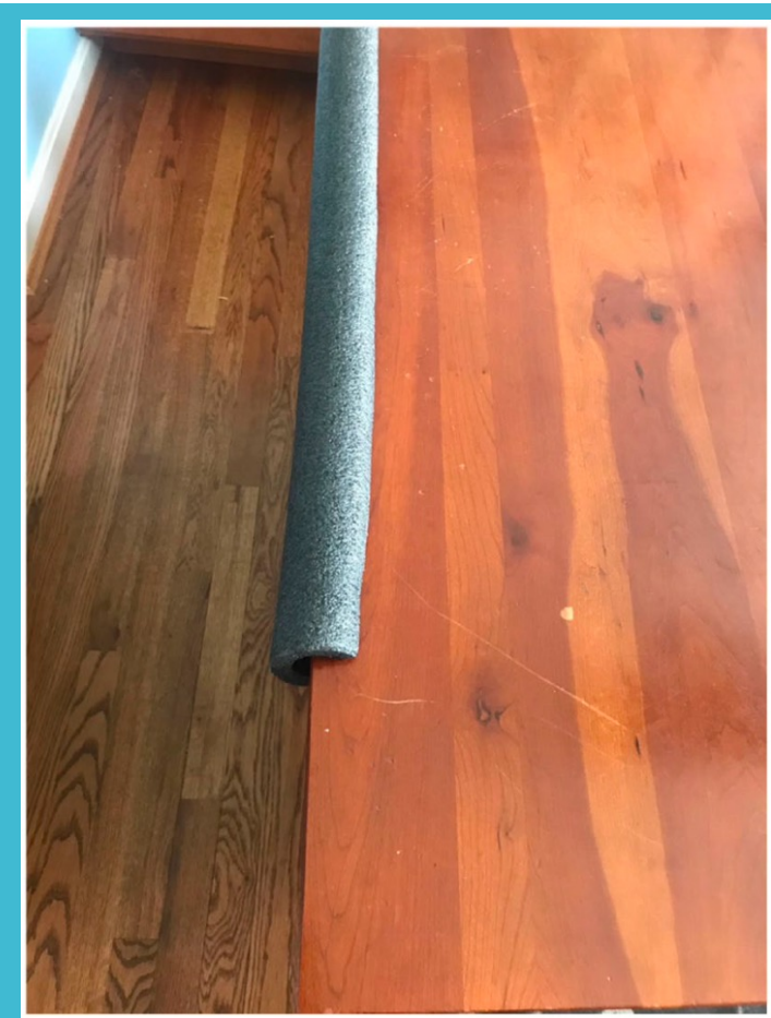
A pipeline insulation used to prevent contact stress
