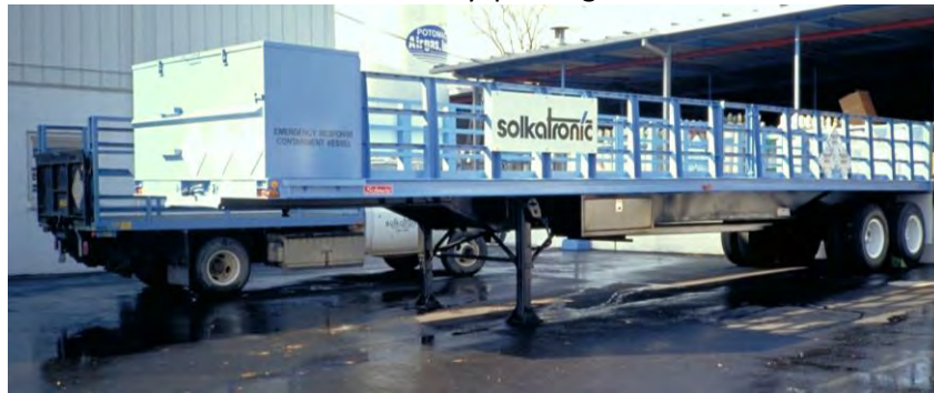
ERCV Enclosure on Cylinder Trailer
