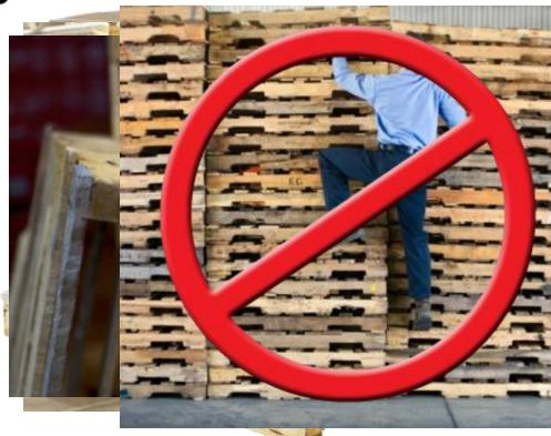
For wood pallets, the pile cannot be more than 6 ft (1.8 m) in height, and for plastic pallets, the pile cannot be more than 4 ft (1.2 m) in height. In both cases, the piles must be separated by a minimum of 8 ft (2.4 m) of clear space or 25 ft (7.6 m) of stored commodity.
