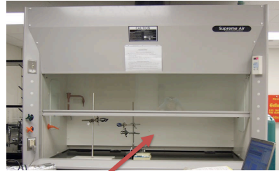
Airflow measured at face of opening with sash positioned at operating height.
