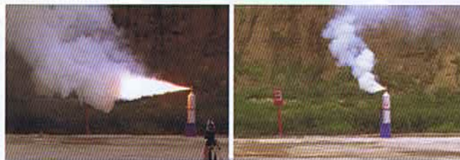
Figures 4 and 5: A silane release from a cylinder valve without (left) and one with a 0.010" RFO (right).
