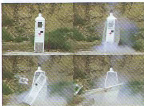
Figures 6-9: A gas cabinet silane explosion triggered during testing.
