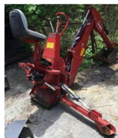
Figure 4 - Excavator (backhoe) attachment involved in the incident
