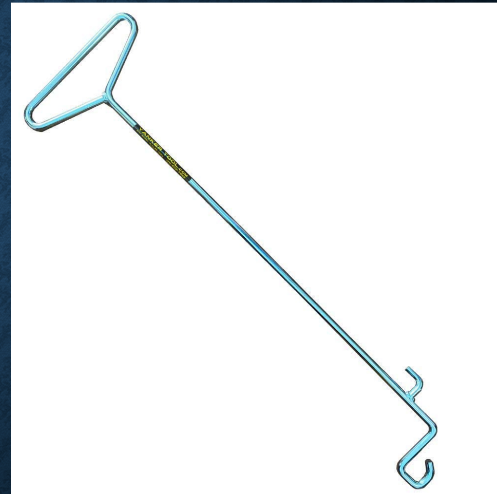
Fifth wheel release safety hook
